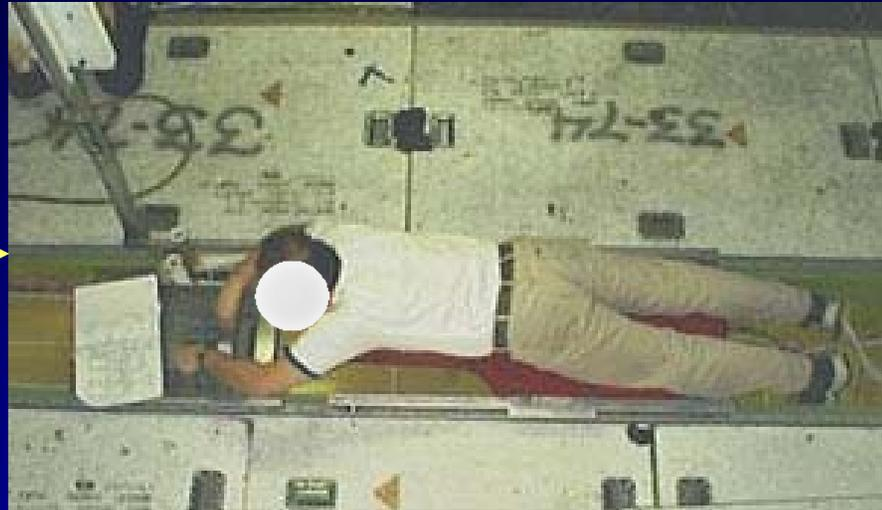
***Access work area from a prone position using a work platform mounted on wheels, for easy relocation along the work area, and having cutouts for arm clearance. In later designs, a head support was added to reduce potential neck strain.***
